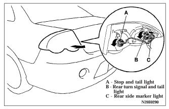
3. Slide the light unit outward to remove it. Remove each bulb socket assembly by turning it counterclockwise. Remove the bulb from the socket by turning it counterclockwise while pressing it inward.
